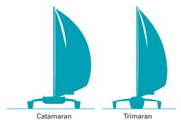
A two-hulled boat is a catamaran. A trimaran has three hulls.
