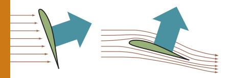
past creates an area of low pressure in front of the fabric and an area of high pressure behind it. The sail is pushed from high pressure toward low pressure, carrying the boat with it. That allows the boat to move with greater efficiency at angles to the wind than otherwise possible with a flat sail.
