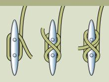
The turns of the line against itself will create enough friction to prevent the line from loosening. A final half hitch thrown around one of the horns will secure the running end of the line. Loosening the line is simply a matter of undoing the half hitch and releasing only enough of the loops to allow the line to run out in a controlled manner.
