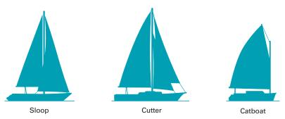
One-masted boats include the sloop, the cutter, and the catboat.
